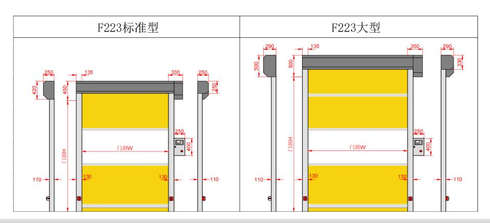
All marked dimensions are only the dimensions required for the product itself, Excluding additional space required for installation and maintenance.
