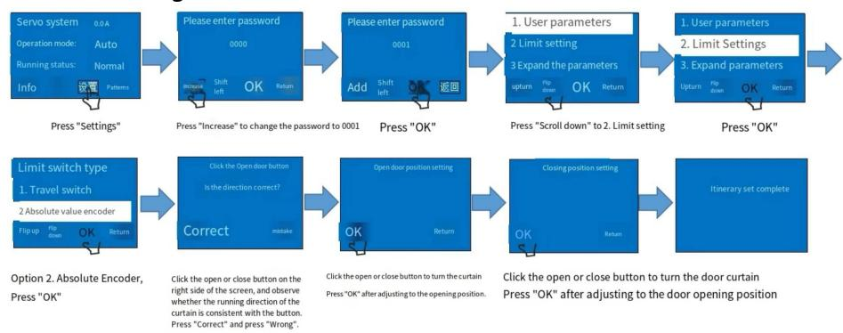
Quick key setting limit (blue SA button in the lower right corner of the controller):
