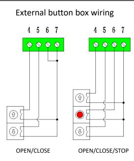
Attention: After pressing the "Stop" button, the door will be in a stopped state, and induction switches are invalid. Only by pressing the "Open" or "Close" button can it resume operation.
